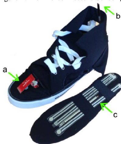
Figure 2: Instrumented Shoe from Smartxa Project: (a) Inertial Measurement Unit; (b) Flexible Goniometer; and (c) Pressure Sensors [2]
